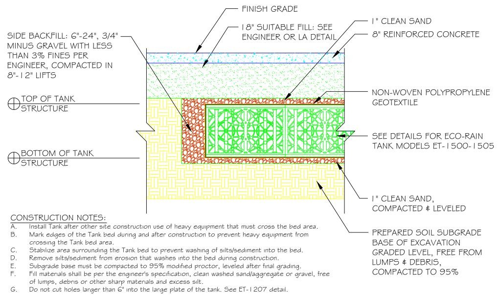
H. Read manufacturer's submittal and use the attached checklist to ensure proper installation.
